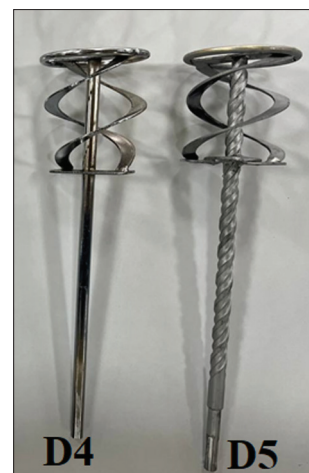
Fig. 7. Helical Stirrer helical stirrer with a cylindrical shaft (D4) and a helical stirrer with a helical shaft (D5).
